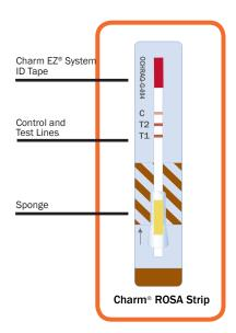
The **Charm® ROSA® Ochratoxin Quantitative Test (OCHRAQ-G)** delivers rapid and accurate results using ROSA (Rapid One Step Assay) lateral flow technology. The diluted extract is applied to the test strip, incubated for 10 minutes, and read in the Charm EZ-M system.
